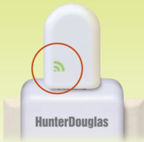
Press and hold the
