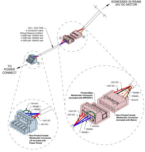
Wiring Distance to Motor • 240ft with 14AWG wire
